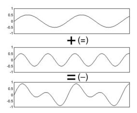
In general, it's possible to break up a complex speech signal into component waves, using technology (typically by doing a Fourier transform)
